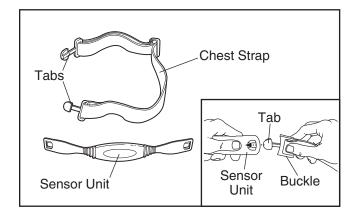
Next, wrap the chest pulse sensor around your chest and attach the other end of the chest strap to the sensor unit. Adjust the length of the chest strap, if necessary. The chest pulse sen-
